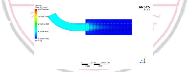
Figure 14 Velocity contour for case 3
